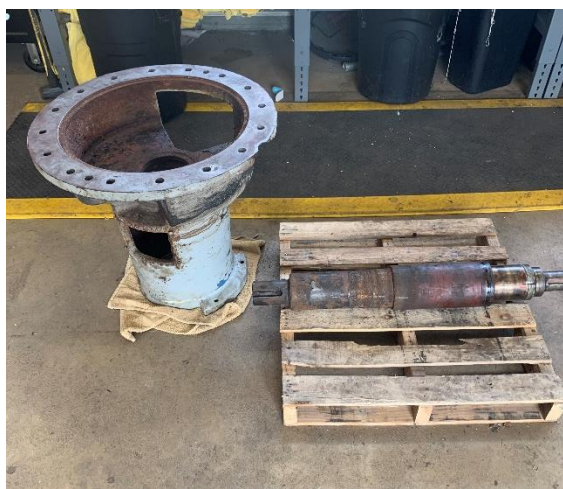
Disassembled Pump and Shaft.
